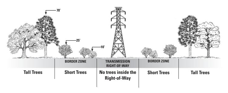
CenterPoint Energy's policy is to remove vegetation that will at some time interfere with the safe operation of our transmission lines. The intent is to produce a low-growing, predictable environment within our transmission line corridors, which has been recognized by the Federal Energy Regulatory Commission (FERC) as a utility model for ensuring safe and reliable operation of the transmission grid.
